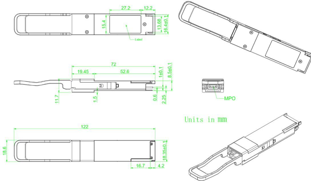
**Figure9. Mechanical Specifications**
