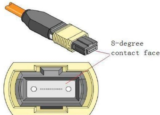
**Female MPO Connector with 8-degree End-face for this module**
