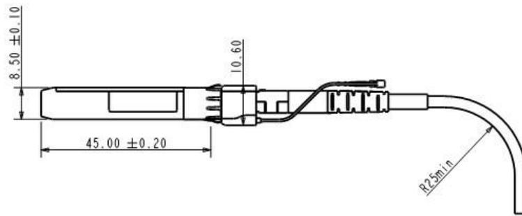
**Figure1. Mechanical Specifications**
